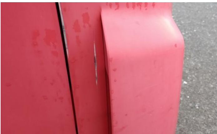
11: Door osf Scratched Over 25mm Thru Paint
