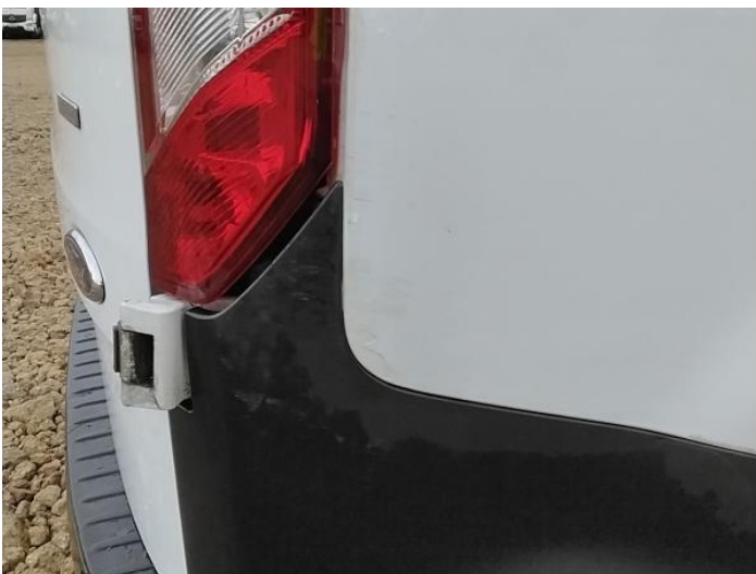
7: Qtr Panel osr Dented With Paint Damage
