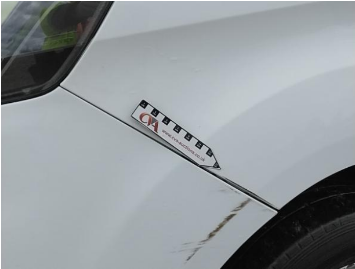
3: Wing nsf Scratched UpTo 25mm Not Thru Paint
