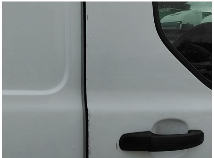
10: Door osf Chipped Edge Chip
